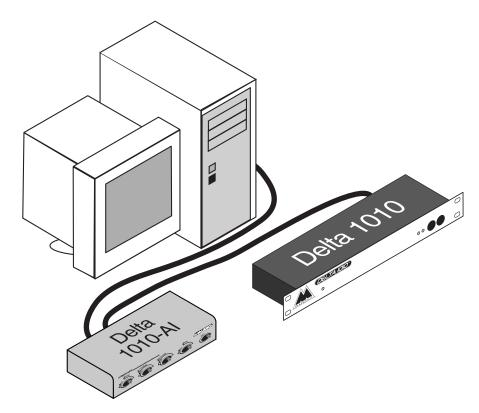
NOTE: If you are using your Delta 1010 solely for optical transfers and do not need A/D or D/A capability, it is not necessary to connect the Delta 1010 rack mount unit. However, synchronization via MTC may be desired, and your Delta system will lose its MIDI function without the rack unit (see section, "Synchronizing Your ADATs").
